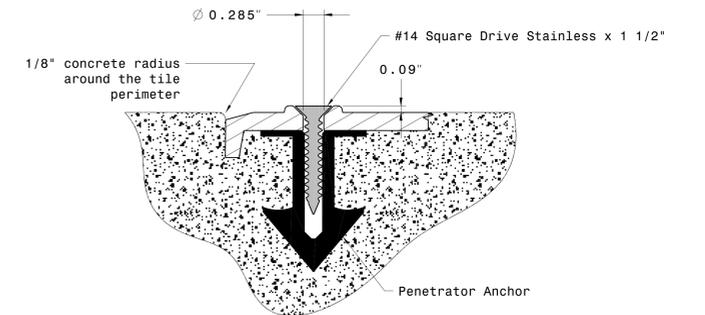
TYPICAL PERIMETER FASTENER DETAIL
